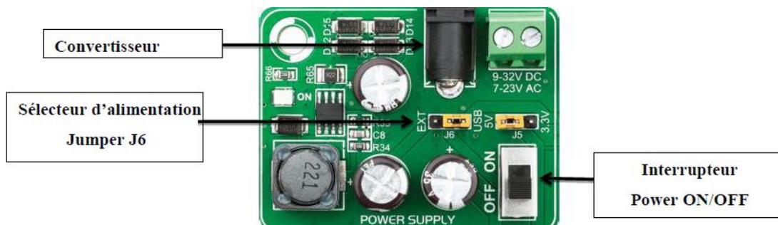
Figure IV.1 Alimentation (Jumper j6 en position USB)
