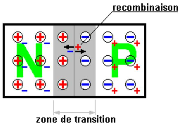
FIGURE 1.8 : FONCTIONNEMENT DE LA JONCTION P-N
