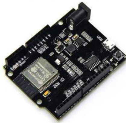
Figure II.4: Carte ESP32 Format Arduino [21]
