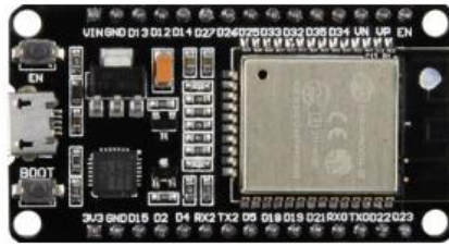
Figure II.3: Carte ESP32 NodeMCU [21]
