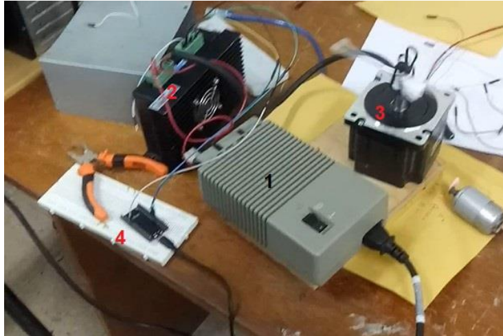
figure 38: fully wired circuit with NEMA34 and ESP32
