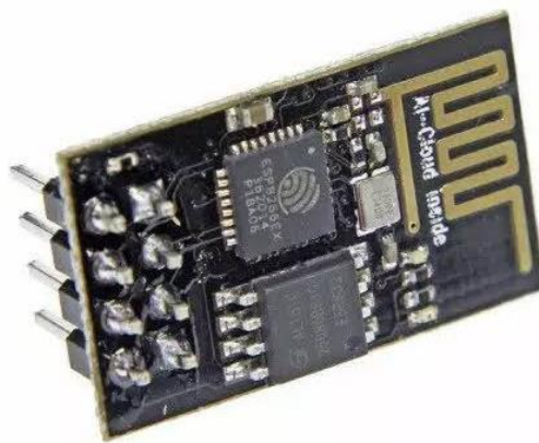
Figure 25 Module wifi esp8266
