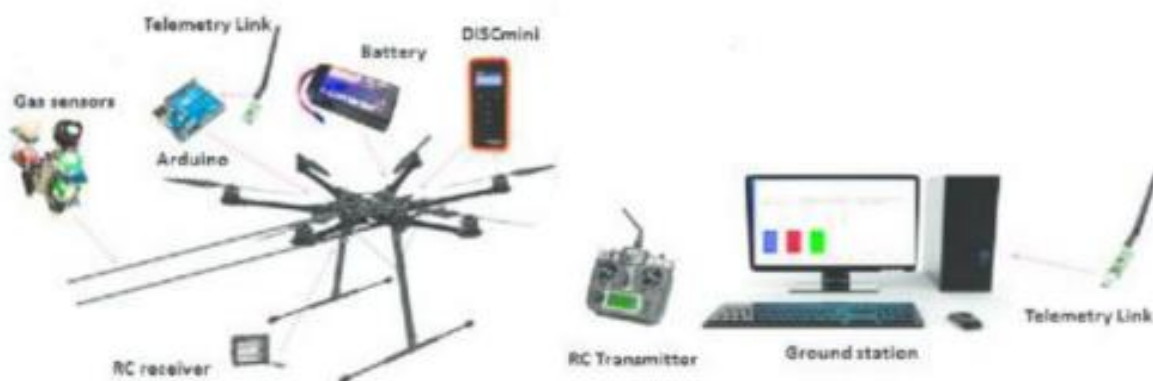
Figure 3.2 : A typical UAS consists of five main components
