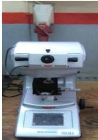
**Figure II-8:**Micro durometre
