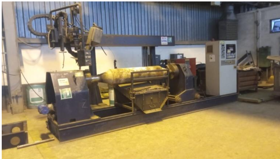
Figure III-2 : la machine (WELD CLAD)
