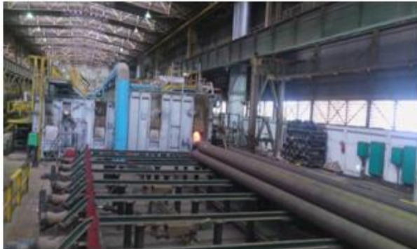
Figure III.5 : Four de trempe
