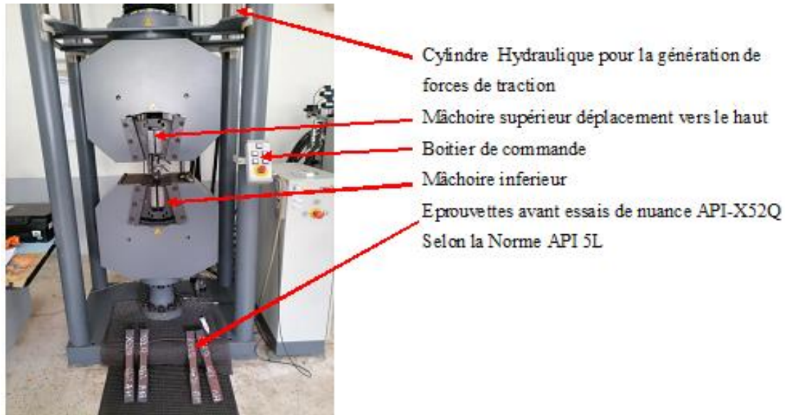
Figure III.21 : Machine de traction Z1200 ZWICK/ROELL 120T°
