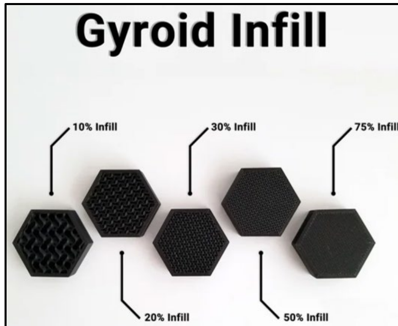
Figure 43. Cut sections with Different % density in gyroid infill pattern.
