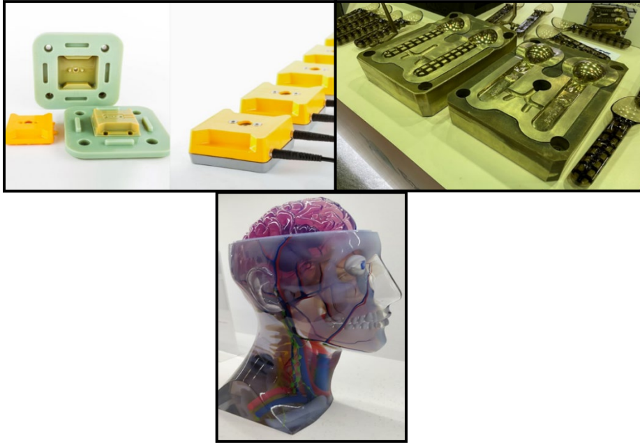
Figure 18. Top Left «Low Run Injection Molded Sensor Housings », Top Right «Steel Base Injection mold» Bottom « Full Model of a human skull »
