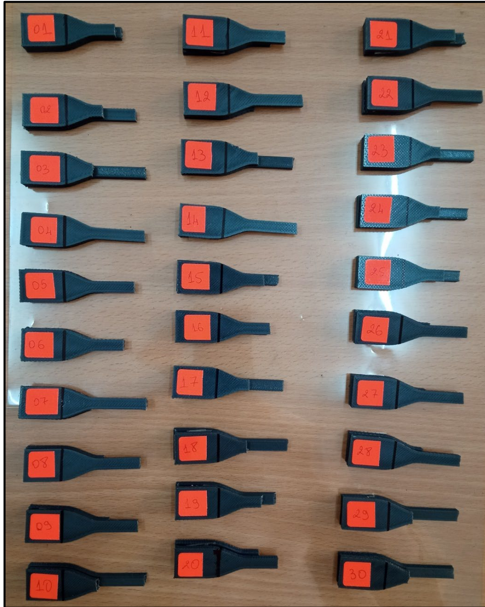
Figure 41. All the printed specimens after the tensile test
