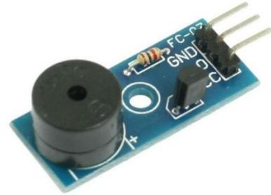
**Fig2.7** LE buzzer
