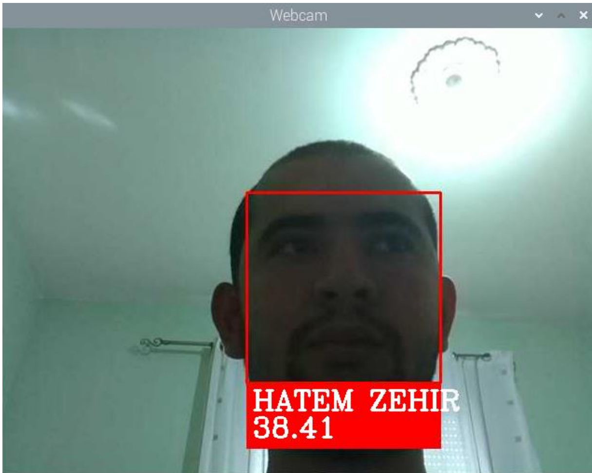
Figure III.2: a red rectangle will be drawn around the face if the temperature is higher than 38°C
