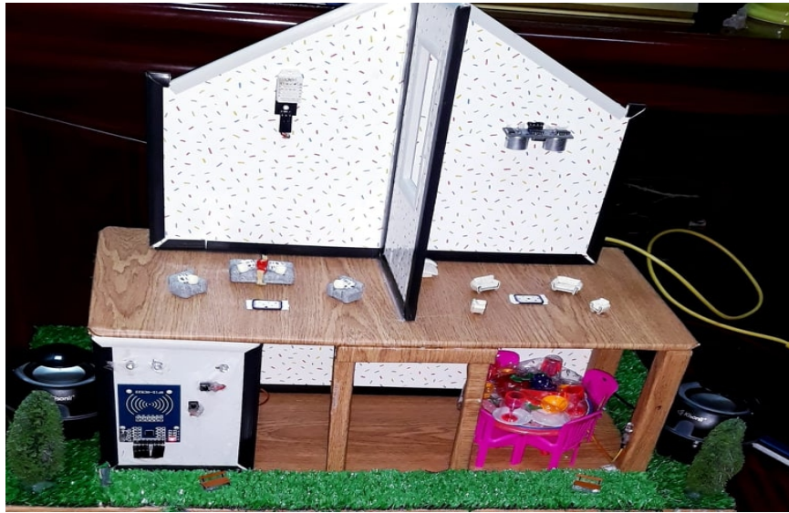
Fig.41. the Smart Home Prototype with the speakers on the side for the voice alerts.
