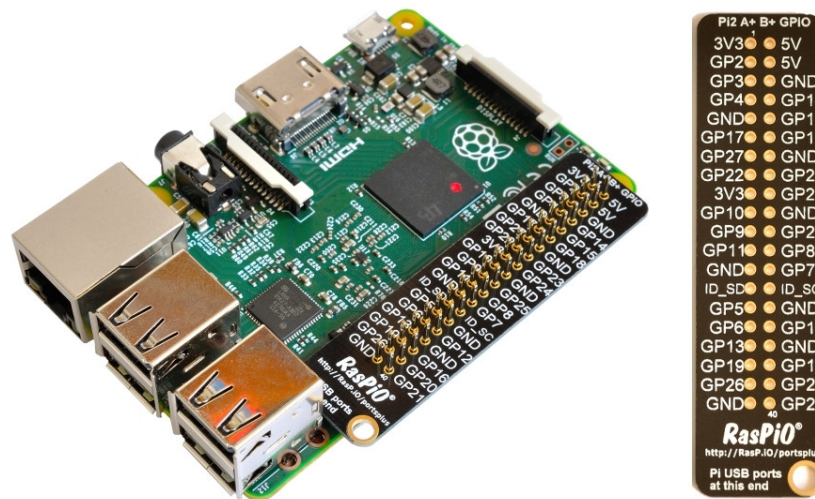
Fig.8. GPIO Pins and Their Functions
