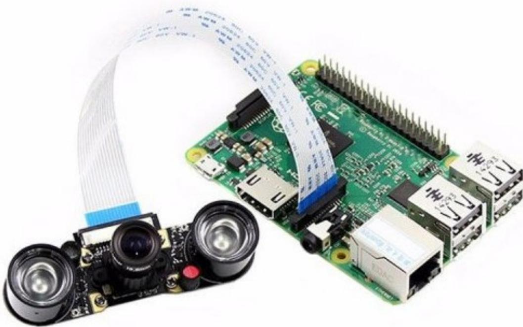
Figure 30: Module camera infrarouge
