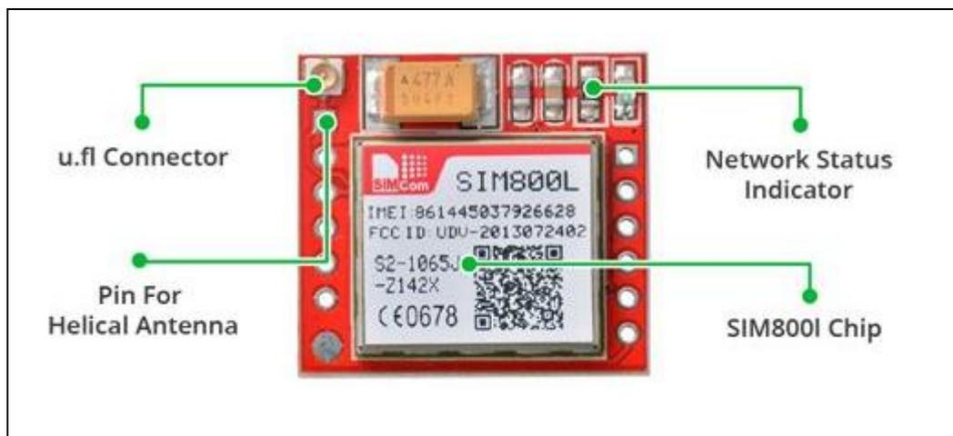
Figure 6: GSM SIM800L
