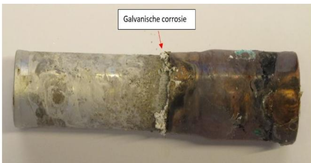
Figure II.1. La corrosion galvanique
