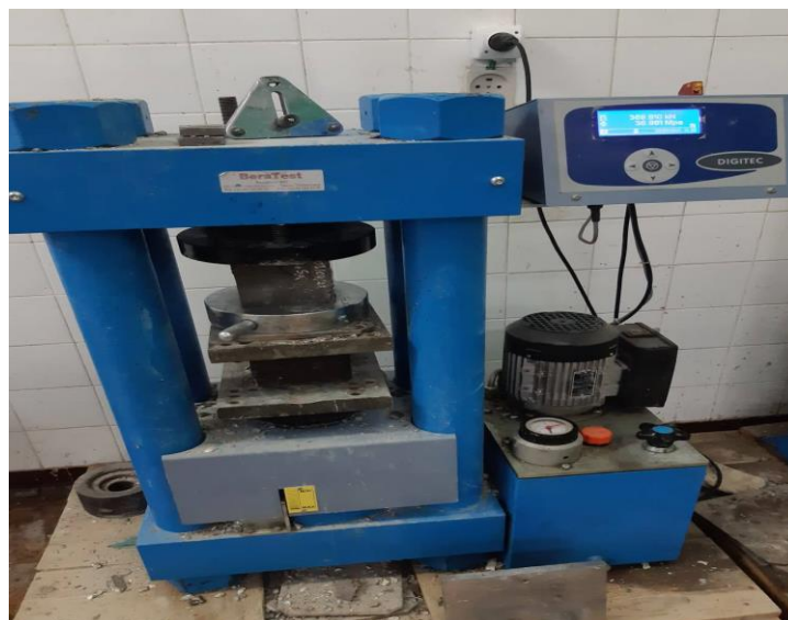
Figure II.31. Essai de compression.
