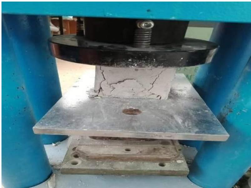
**Figure II.13** :Essai de compression.
