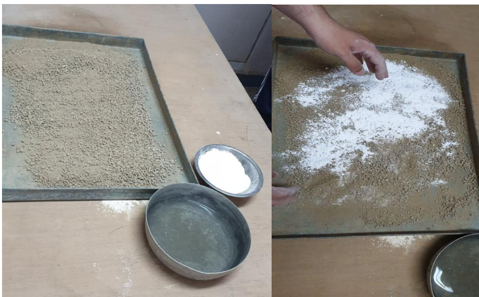
Figure II.28 : Mélange argile + la chaux
