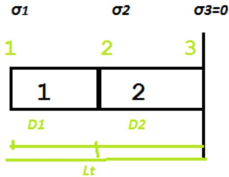
$$\sigma_{tmb1} = \frac{\sigma_1 + \sigma_2}{2} \quad \sigma_{tmb2} = \frac{\sigma_2 + \sigma_3}{2} \quad D_{max} \leq \left(\frac{2}{3}\right) * L \leq \left(\frac{H_{etg}}{2}\right)$$
