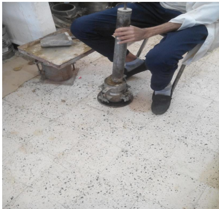
Figure 3.2 : essai de compactage
