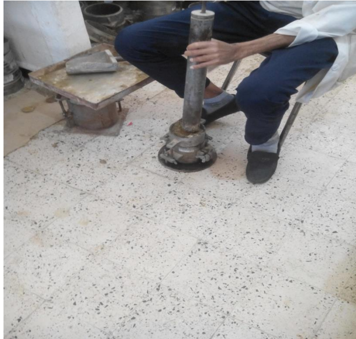
Figure 4.2 : Essai de compactage
