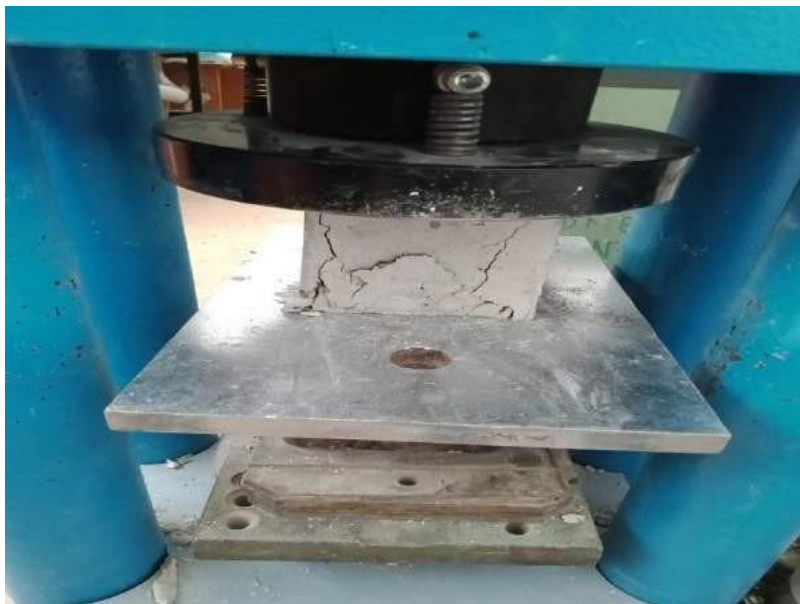
Figure II.13 : Essai de compression.
