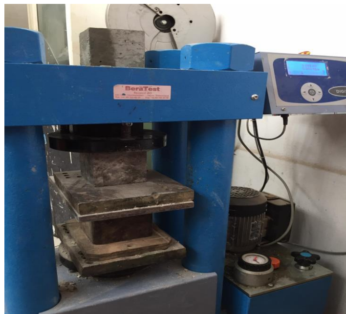
Figure III-1 Essai de compression
