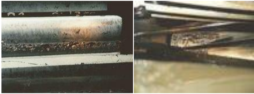
Figure III.9 : Ecaillage des dents
