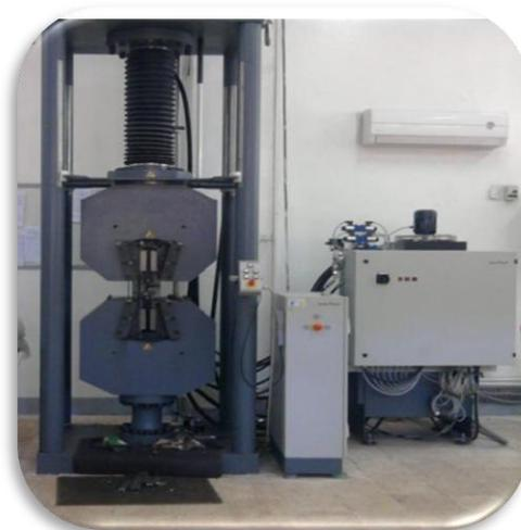
**Figure I.2** la machine de traction.
