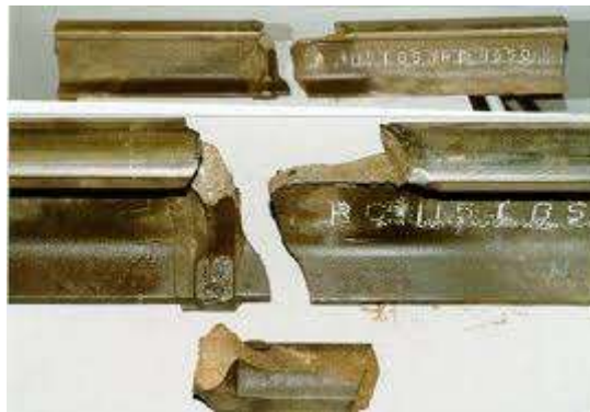
Figure II.23: Rupture des rails
