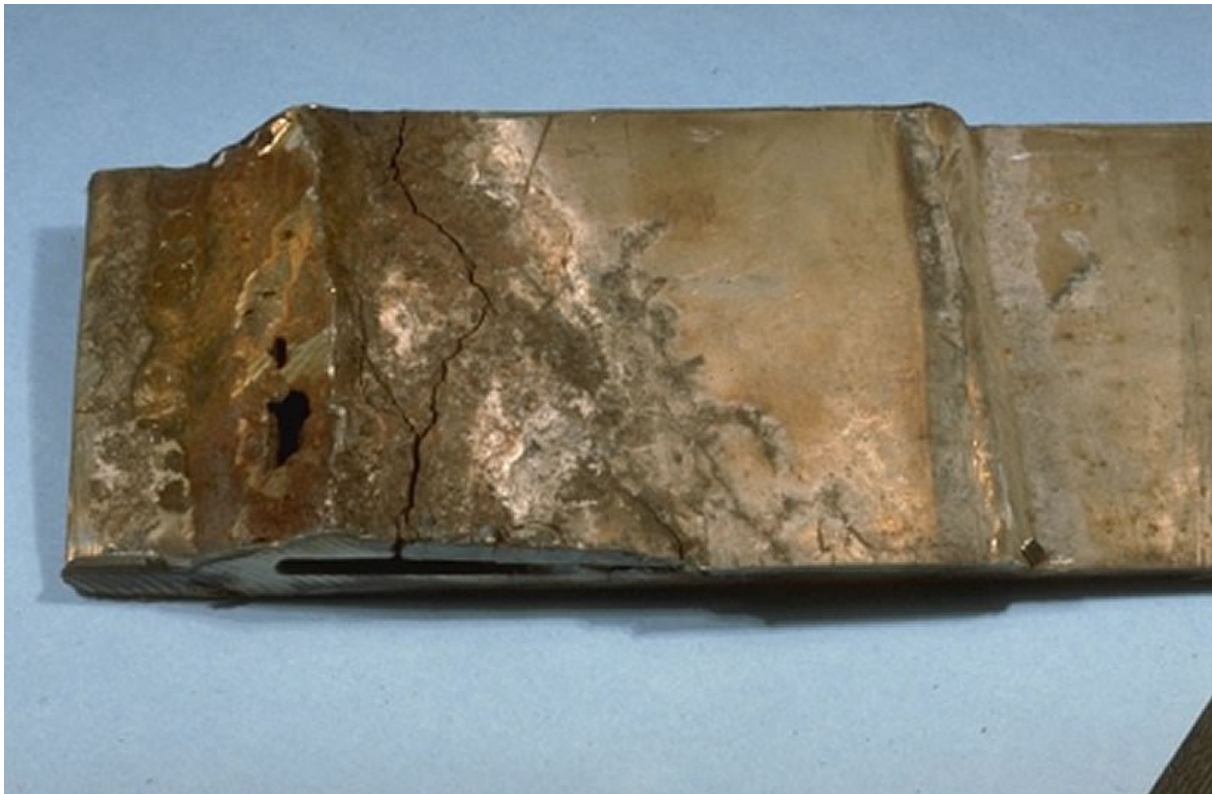
Figure 14 Stress corrosion cracking in a welded alloy steel structure (stresses induced by welding) [3].
