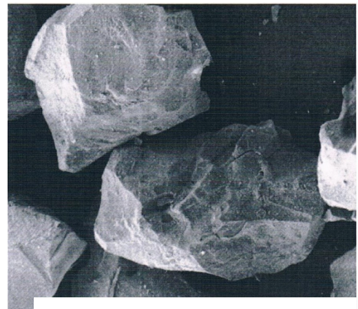
Figure 3: Sable d'olivine (x75)
