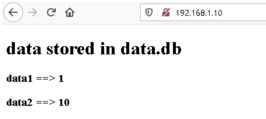
Fig III.6- result of the web application using flask and Sqlite3
