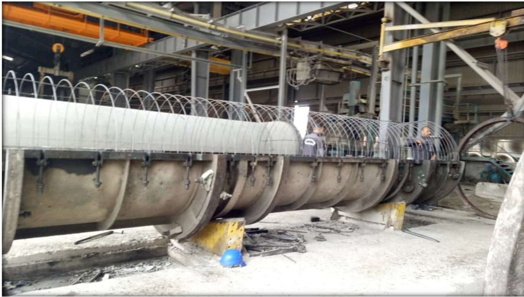
Figure 22-insertion de la cage d'armature minimale
