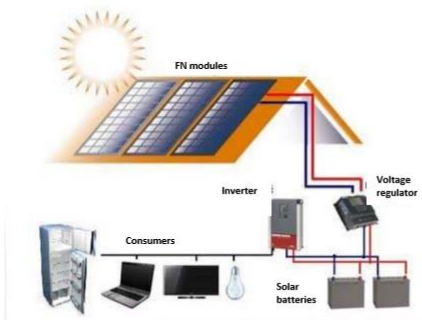
Figure 2.17 Standalone photovoltaic system
