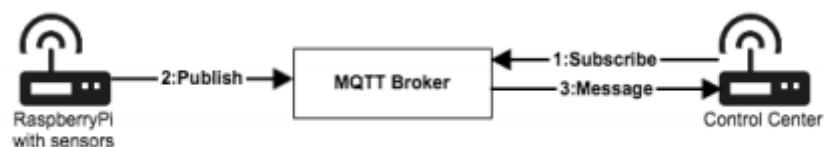
Figure 20 : Architecture MQTT « publish/subscribe »
