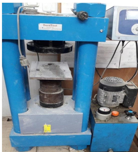
Figure IV.6 : Machine de compression
