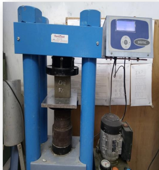
Figure II.11: essais de compression simple
