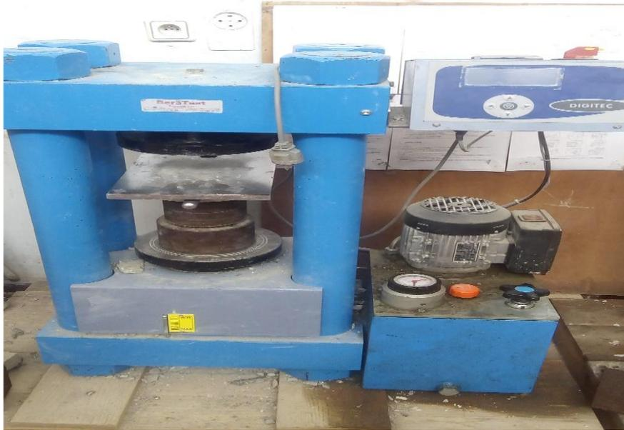
**Figure (III-5) :** essai de compression
