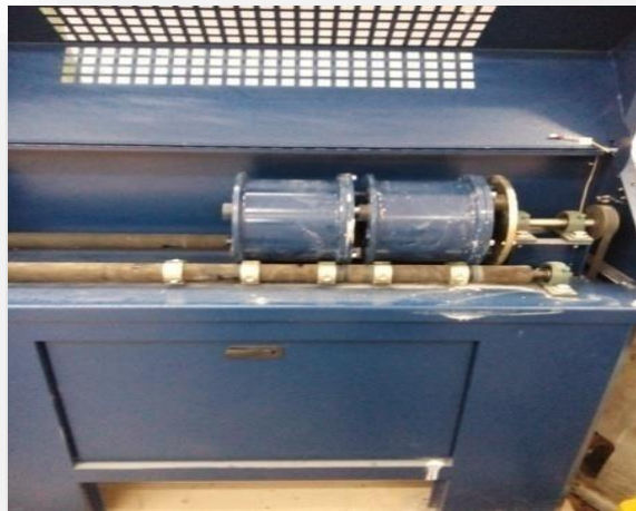
Figure II.8- Essai de micro Deval
