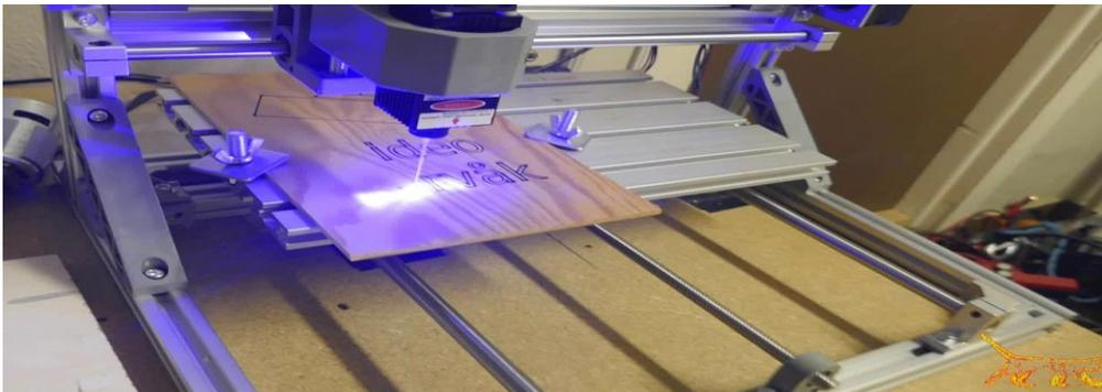
**Figure I. 8 :CNC 3018 Engraving Machine 5500 mw laser**
