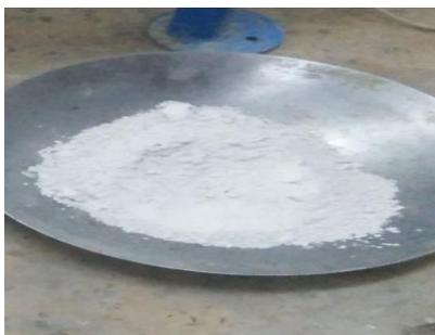
**Figure II.5.** Filler de calcaire
