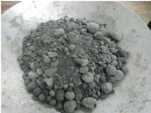
**Figure II.3.** Clinker
