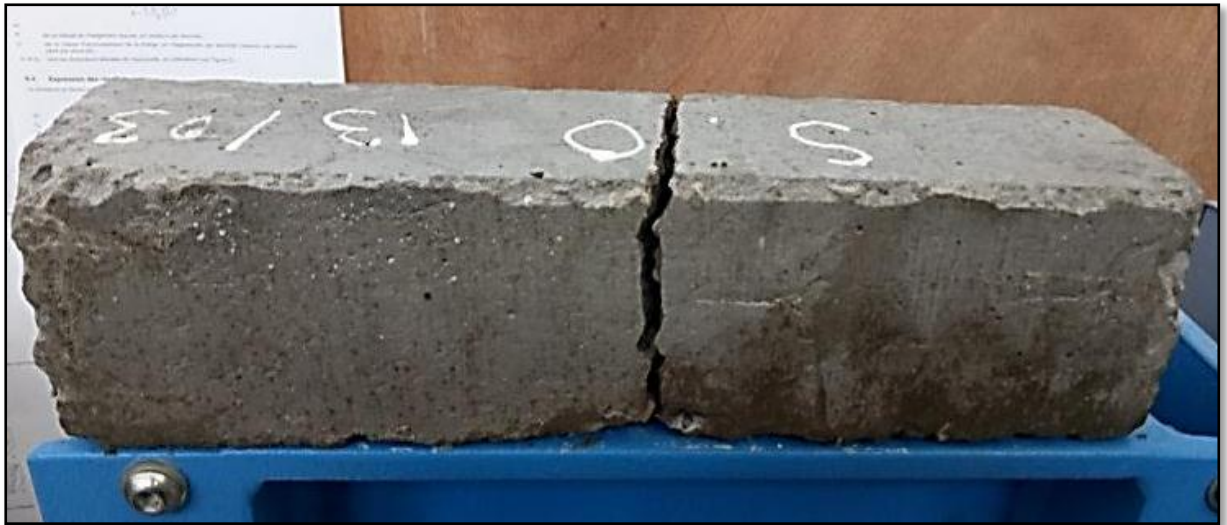
Figure III.12 : Rupture centrale droite.
