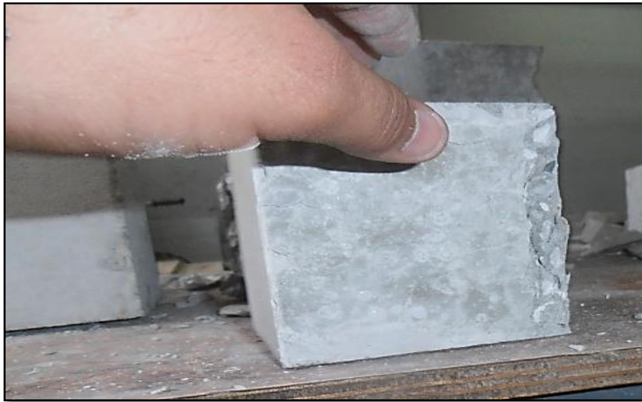
Figure III.10: Exemple de rupture incorrecte.
