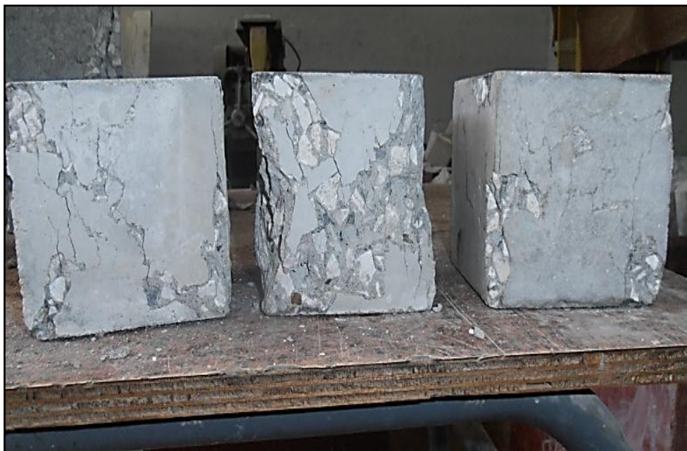
Figure III.9: Exemple de rupture correcte.
