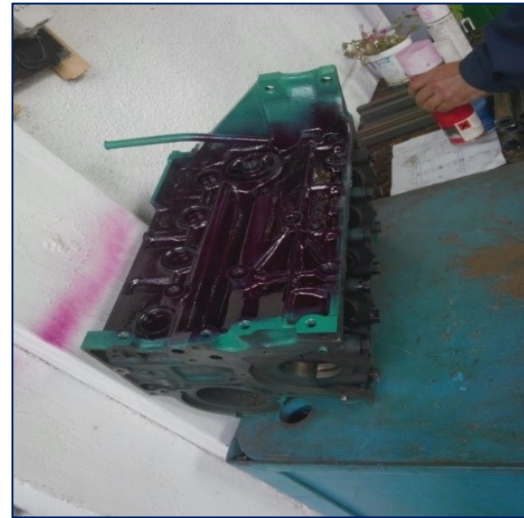
Fig. 4.10. Application of the penetrant
