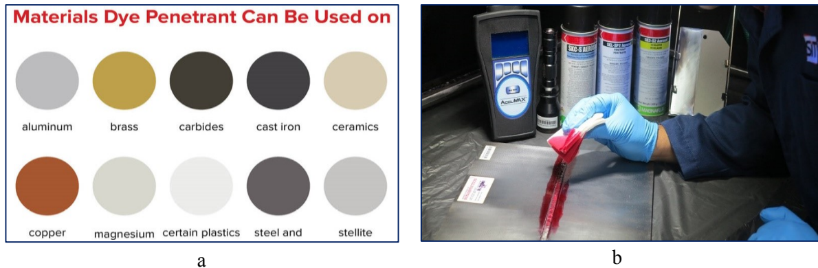
Fig. 3.1. Liquid Penetrant Materials and Application [88] [89]
