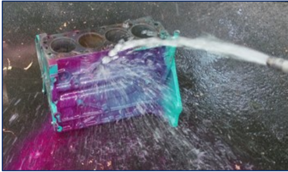
Fig. 4.11. Removing the penetrant excess
