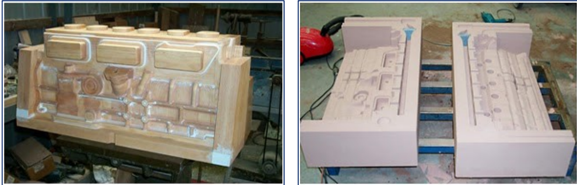
Fig. 4.7. Casting Engine Block [128]
