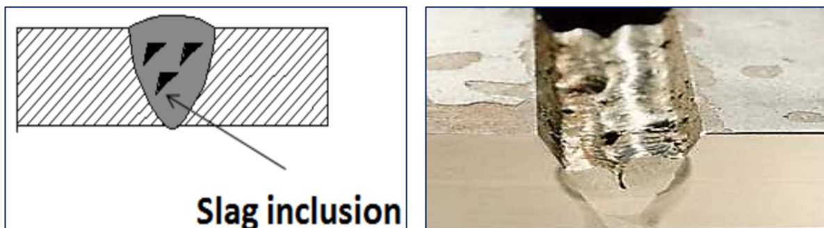
Fig. 2.10. Smooth weld bead profile allows the slag to be readily removed between passes [55] [71]
