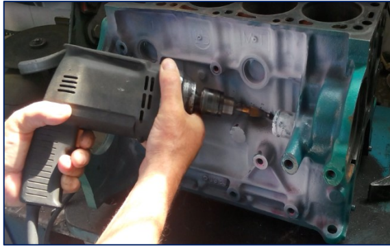
Fig. 4.14. Performing the “V” groove
