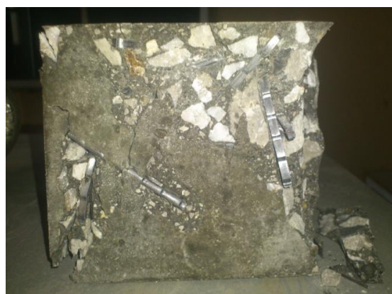
Figure III 5. Mode de rupture en compression.
