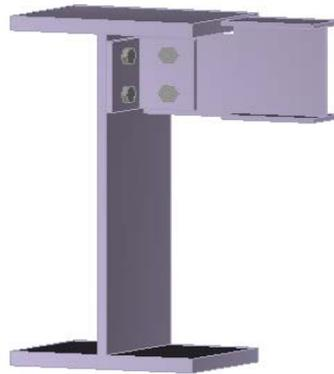
Figure VIII 1: Assemblage solive-poutre principale.
