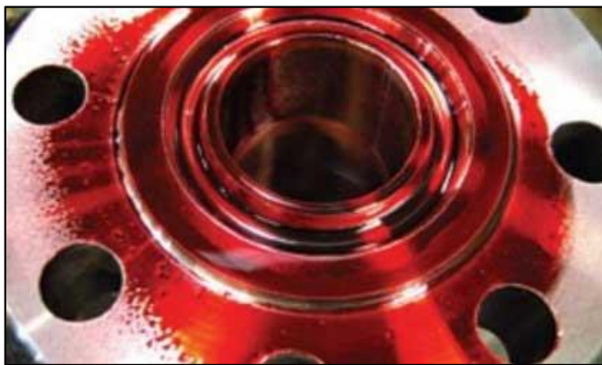
Fig 2.26 Liquid Penetrant Testing [98]
