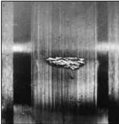
Fig.2.2 The progression of surface rolling contact fatigue [31]
