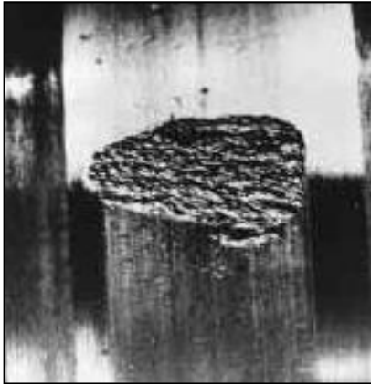
Fig.2.4 The progression of surface rolling contact fatigue [31]
