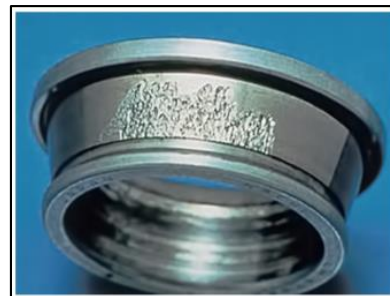
Fig.2.9 Advanced subsurface spalling in a tapered roller bearing
