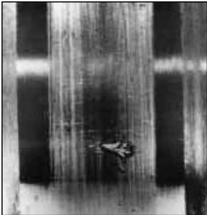
Fig.2.1 The progression of surface rolling contact fatigue [31]
