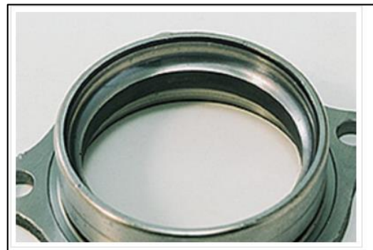
Fig.2.7 Outer ring of double row angular contact ball bearing (rub unit bearing).
