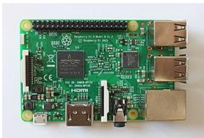
Figure V.2 : Raspberry Pi 3, B
