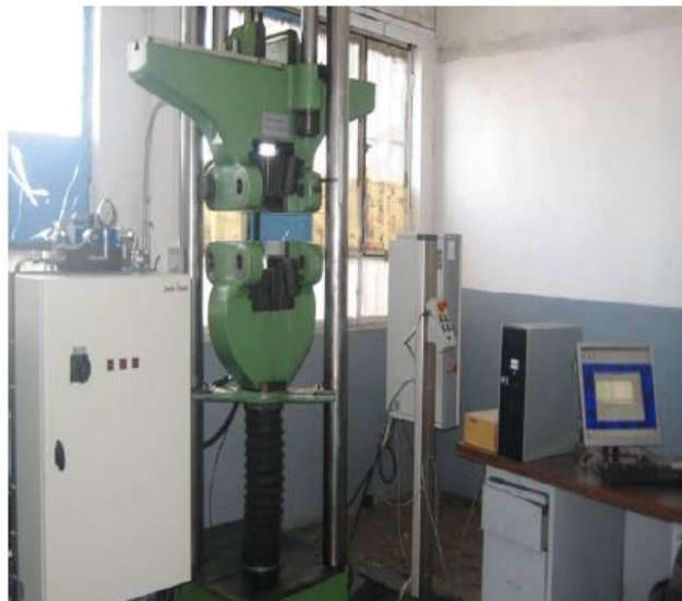
Figure II- 5 : Machine de traction 100T de type Wolpert.
