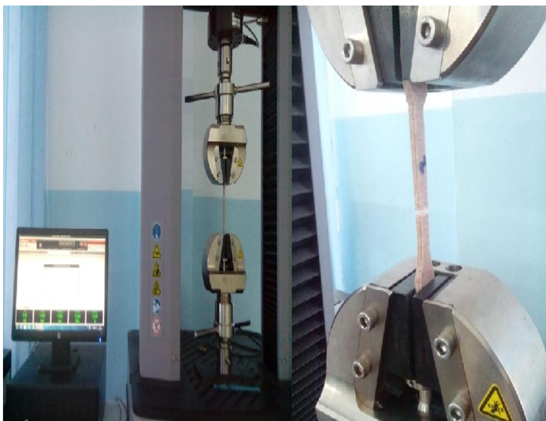
Figure III-5 Machine de traction MTS 43 [25]
