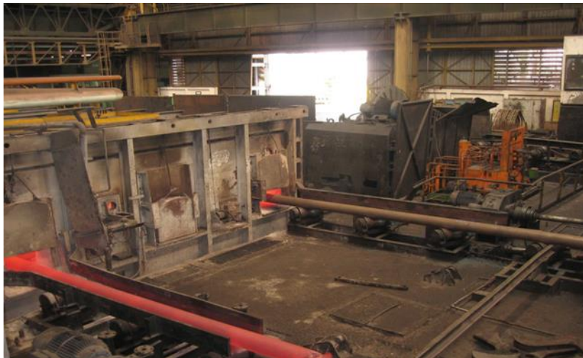
Figure II.1.7 Four à longerons
