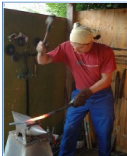
**Figure I.28 :** forgeage libre au marteau manuel. [21]
