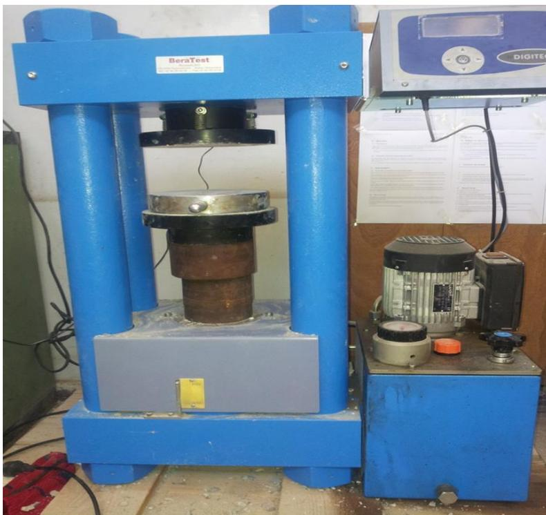
Figure III. 18- Essai de compression
