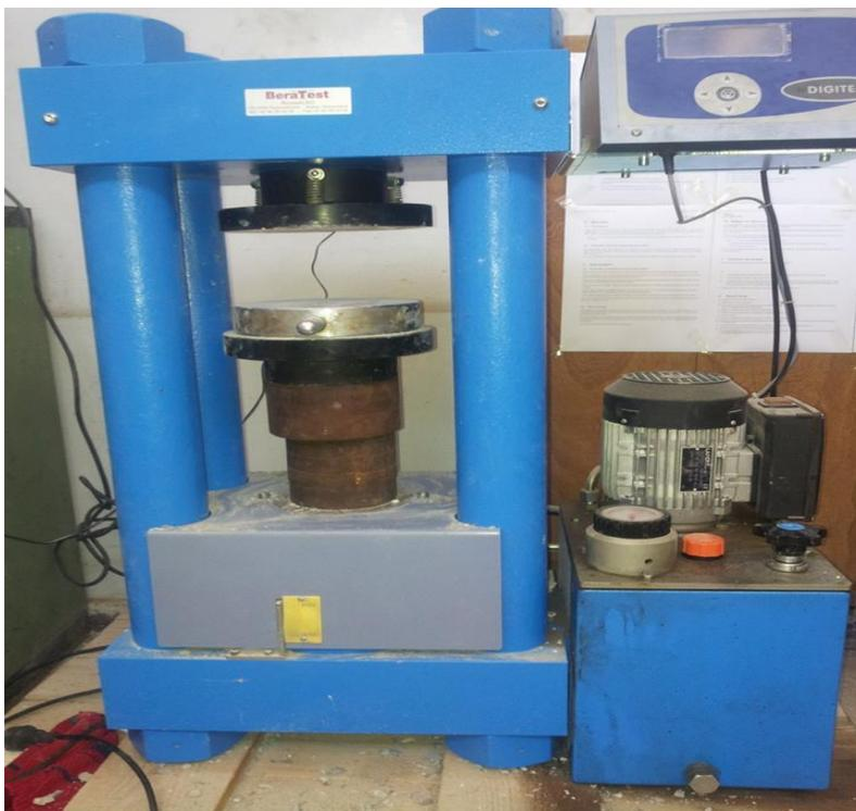
Figure III. 18- Essai de compression
